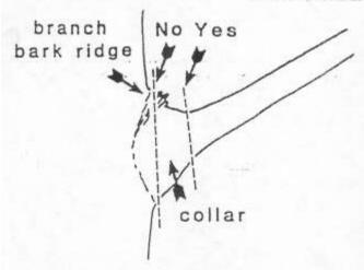
When removing a branch, always cut outside the branch bark ridge and collar. Do not make a flush cut.
